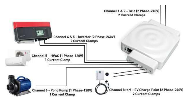
Example of Smappee Setup with CT connection with a 2-Phase (240V) solar circuit, EV charge point and a 1-Phase (120V) pond pump, HVAC installation and submetering.
