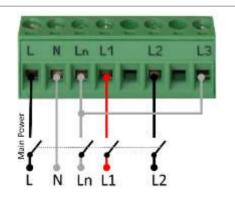
Hints: When no auxiliary power supply is used, you can create branches using wagos for voltage wiring.
