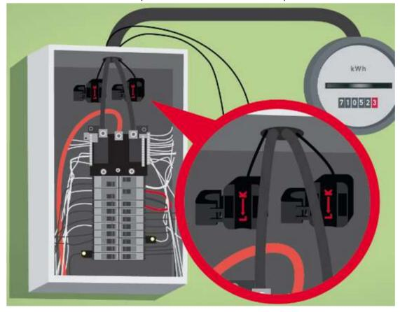
2. Mount the current clamps in correct direction around the power cables
