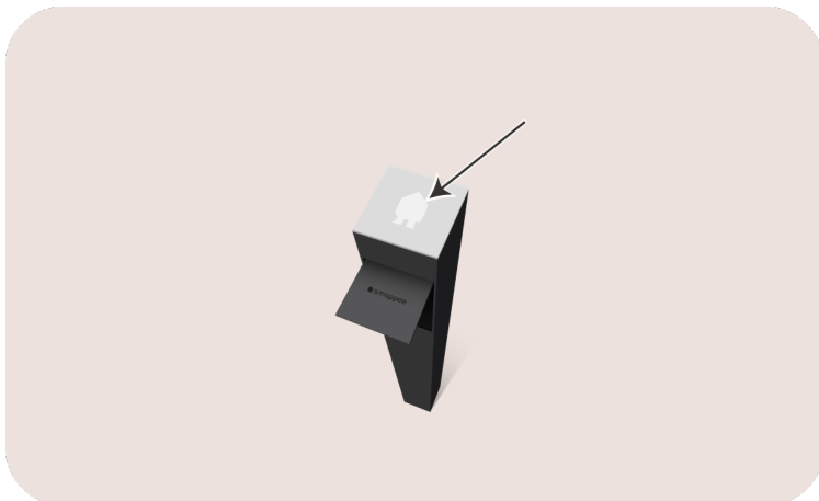
Image 29: Position of the RFID reader with LED on the EV One
