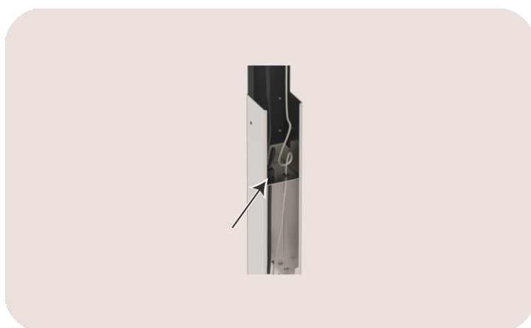
Image 19: View on the holes for the cable entry
