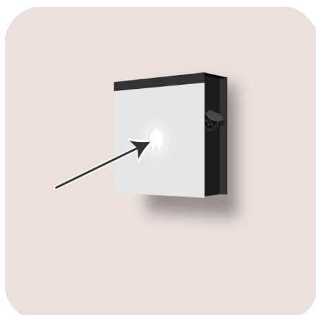
Image 18: Position of the RFID reader with LED on the EV Wall
