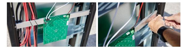
The inverters in the back have the DC output at the bottom of each slot, while the inverters in the front have the DC output at the top.
