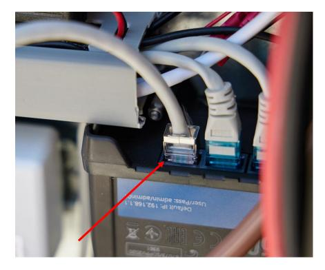
The Teltonika router creates a small, private network within the EV Base Ultra to provide network connectivity for all components. This private network is created within the subnet 192.168.37.0.
