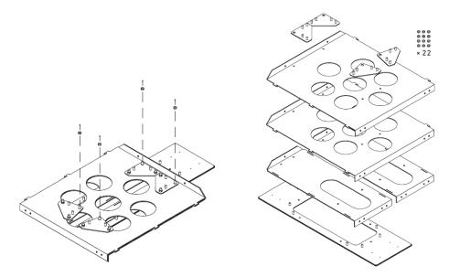
• Join the 4 side panels using the grooves. Hand tightening the 4 mounting corners at the bottom of the assembling using the supplied nuts.
