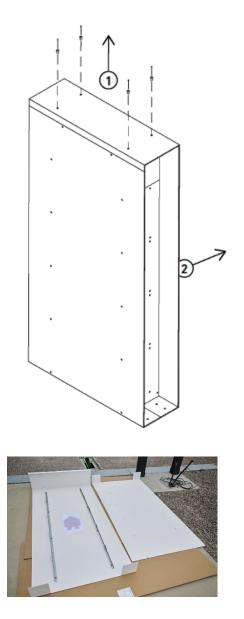
d. A top plate of the EV Base Ultra anchor is already mounted to the charging unit for easy installation. In order to place the EV Base Ultra on the installed anchor, first remove the dummy top plate of the installed anchor.
