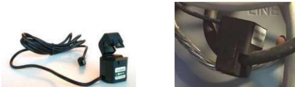
Use one CT on each phase of the load and ensure it has a rating equal to or greater than the breaker rating protecting the circuit (i.e. 200A CT for a main circuit with a 200A breaker rating). Then plug the other end of the CT into the corresponding inputs (1-9) on the Smappee Plus monitor.
