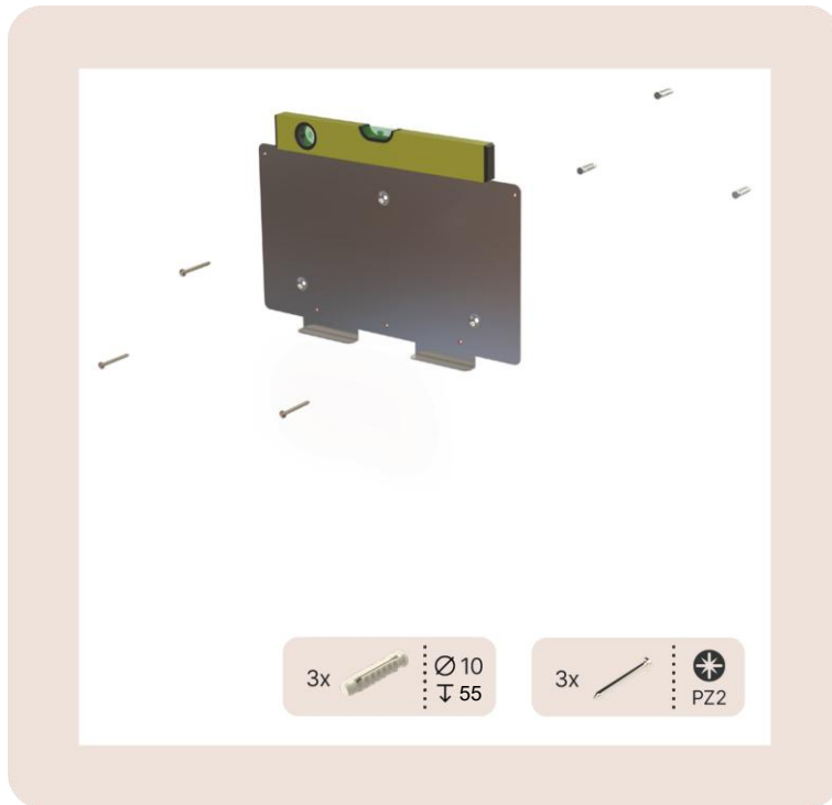
Image 25: View on the wall mounting plate (A) and a spirit level (B)
