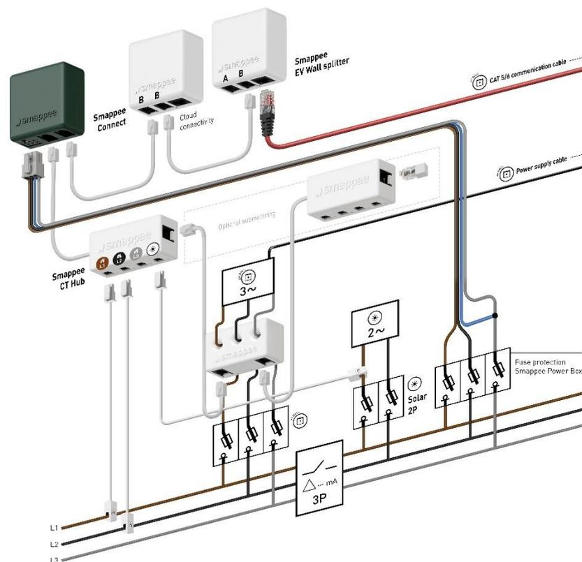
Note that when you measure single-phase loads or solar panels, you must connect and configure the CT(s) as shown below:
