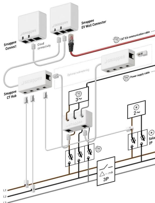
Note that when you measure single-phase loads or solar panels, you must connect and configure the CT(s) as shown below:
