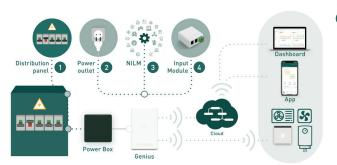
Or, use the Smappee Input Module to count pulses of sensors, meters and other devices or to monitor state changes (low/ high) to trigger other processes. Dynamic load balancing for optimised self-consumption and overload protection - all in one single system.
