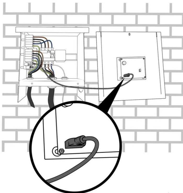
c. Mount and tighten the supplied M4 nuts
