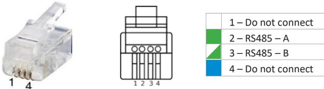
**Note:** The unused wires of the network cable remain unconnected. When a Genius unit is used, connect the RJ10 Splitter (supplied) to the unit.
