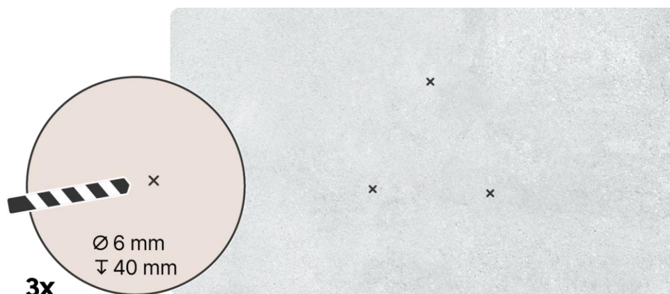
Image 9: Drill holes for the mounting plate
