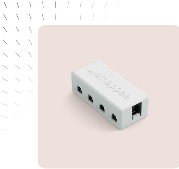
The CT Hub is the main component of the Smappee Infinity monitoring system. You can connect up to 4 Current Transformers (CTs) or Rogowski coils to a CT Hub to measure different currents up to 10,000 A. This allows for accurate submetering of (a group of) appliances. Daisy chain several CT Hubs to measure different installations up to a distance of 100 meters (109 yards).
