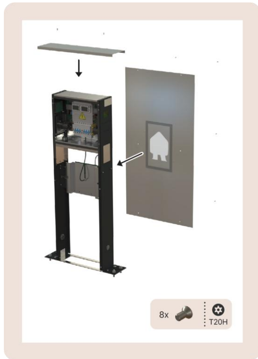
Image 22: View on the top plate (A) and front plate (B)
