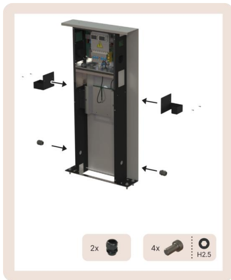
Image 15: View on the pedestal (A) and plugs (B)
