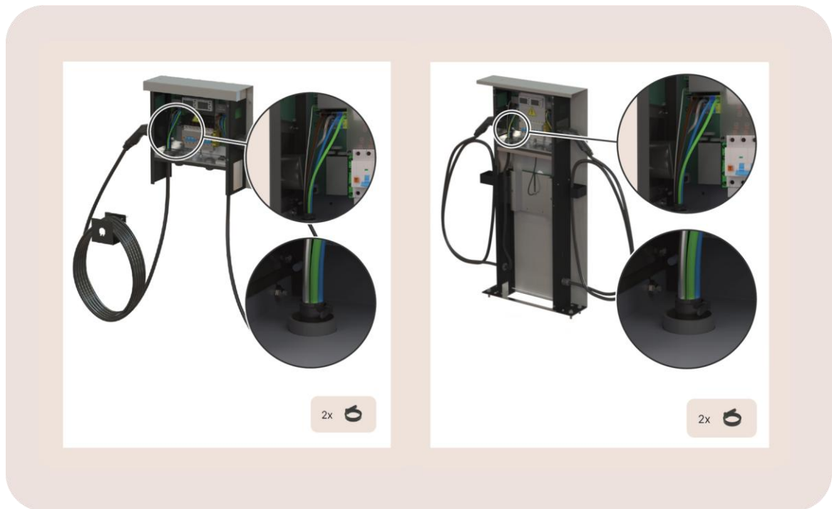
Image 34: View on the cable connections for a wall mounted and ground mounted EV Dual
