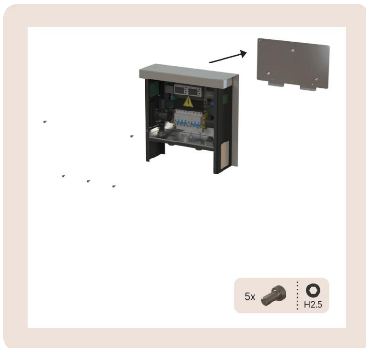
Image 25: View on the wall mounting plate (A) and the EV Dual Core (B)
