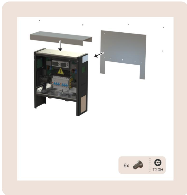
Image 24: View on the top plate (A) and rear plate (B)
