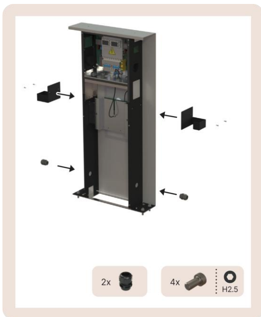
Image 14: View on the pedestal (A), cable holders (B) and cable glands (C)
