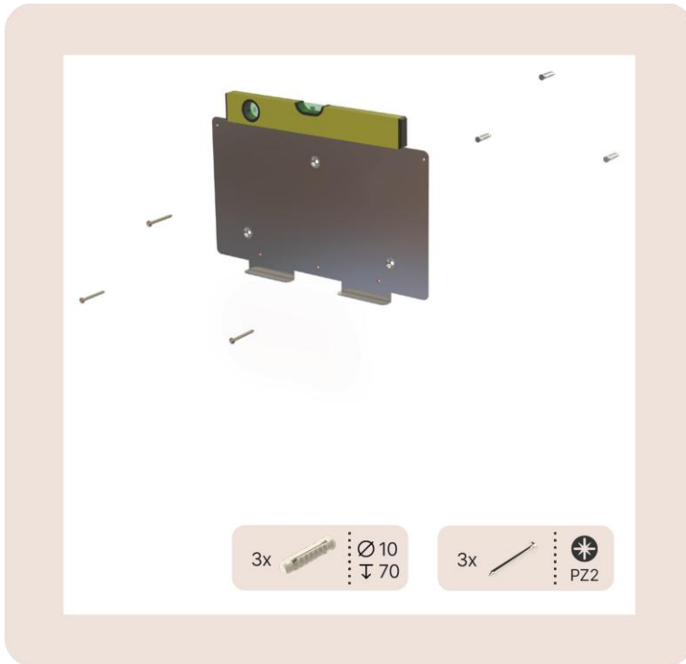
Image 23: View on the wall mounting plate (A) and a spirit level (B)
