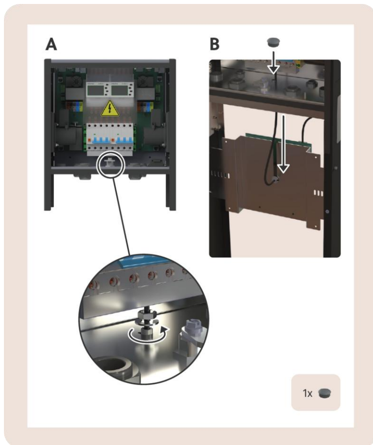
Image 21: View on the antenna removal (A) and attachment to the LED holder (B)
