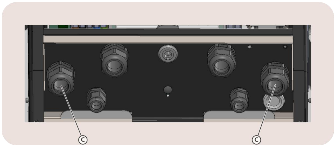
Image 31: View on the cable glands for the charging cables (C).
