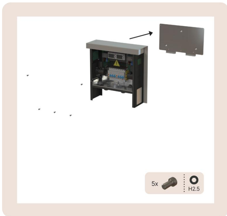
Image 27: View on the wall mounting plate (A) and the EV Dual Core (B)
