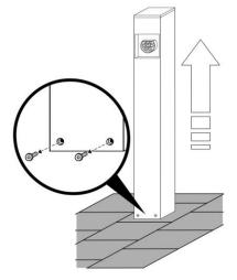
c. When installation is spread over time or there is a risk of damaging the electronics while mounting the EV One, we advise to temporarily remove the top half of the EV One and set it aside in a safe location. To do so, unscrew the four nuts uniting the two parts of the inner structure. No wires need to be disconnected, nor components removed.
