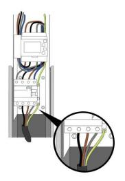
We highly recommend that you test compatibility with the customer's EV during installation. If you have connected the EV One Business as shown above but the EV will not charge, you can try to disconnect the L2 cable going to the socket.
